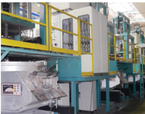
Fig. 1: Transfer of the aluminium alloy into the low-pressure casting furnace
