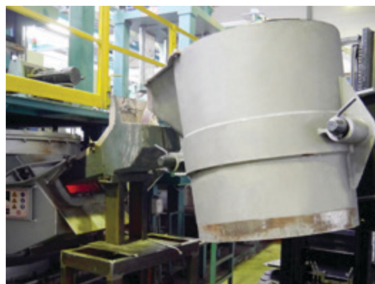
Fig. 2: amTec low-pressure casting furnace with the new heating system
